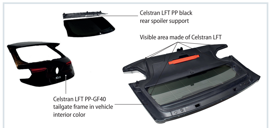
Fig. 4. Since the demands on the tailgate and rear spoiler support differ, they were produced using different materials. Source: A2MAC1; graphic: © Hanser
