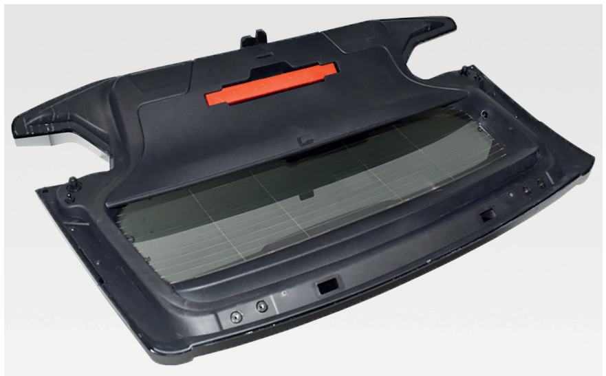
Fig. 2. One part of the tailgate is a visible interior part. The FRP used have a very good surface quality and therefore do not have to be additionally painted. They are supplied as pre-pigmented pellets in the desired vehicle interior color. © Celanese
